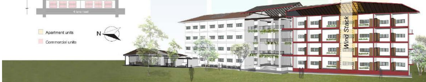
Figure 4.1-14 Features of 5-floor workforce apartment
