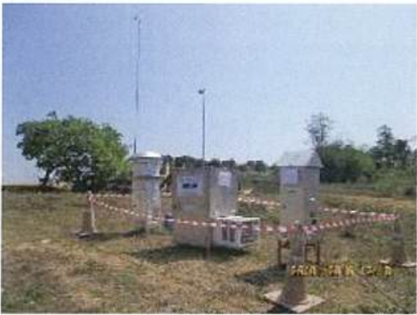
Equipment for Wind and Air Quality Data Collection at Station 2: Myitta Base Camp
