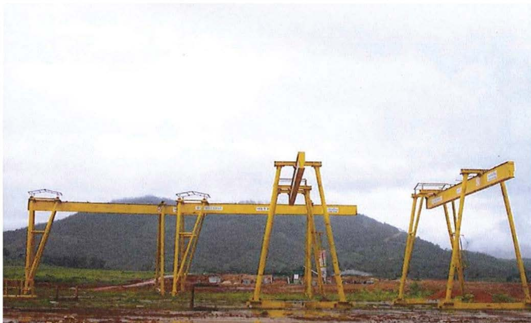
Figure 4.2-2 Precast Construction Equipment
