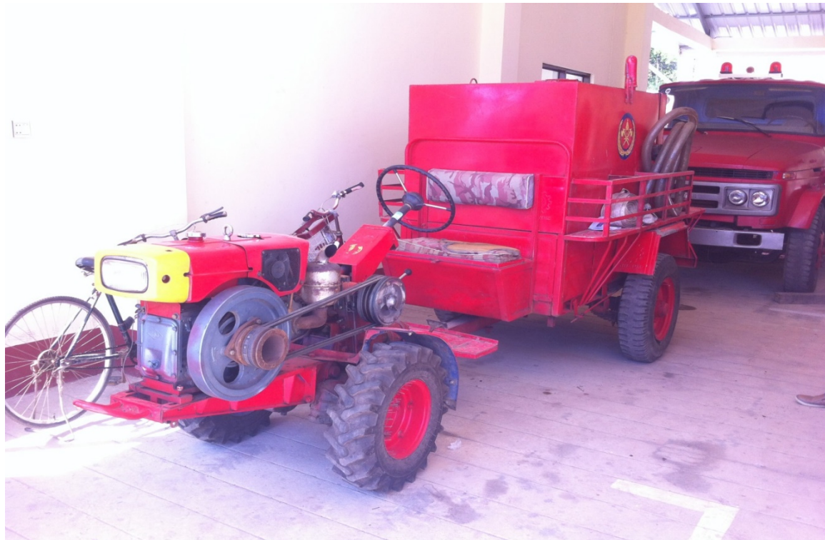
Figure 4.1-51 Yebyu Fire Tank Truck and Fire Tank Tractor (No5 and No.6)
