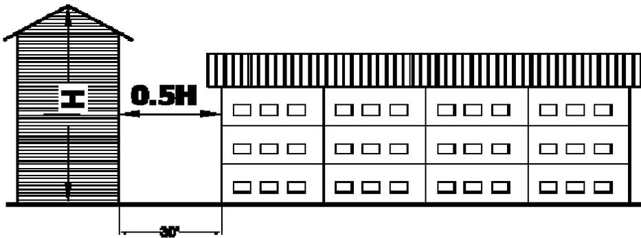
Figure 2.11.2 Schematic Figure Showing Spacing of Row Blocks,
