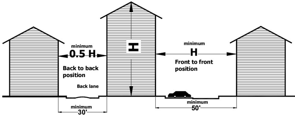
Figure 2.11.1 Schematic Figure Showing Spacing of Row Blocks,
